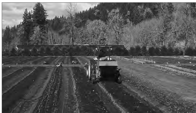
A top-dressing of \frac{1}{4} to \frac{1}{2} inch of ripened biodynamic compost is applied to the beds for perennial plants each spring. Utilizing this mulcher attachment, eight to ten acres of perennial beds can be top-dressed in one day.
