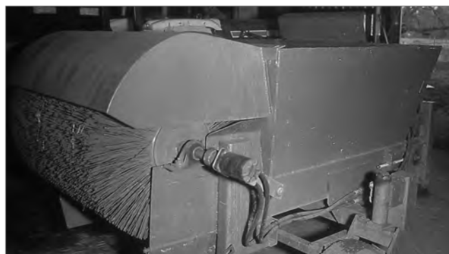
This PTO driven mulcher attachment with a brush that finely crumbles compost was designed by the author several years ago.
