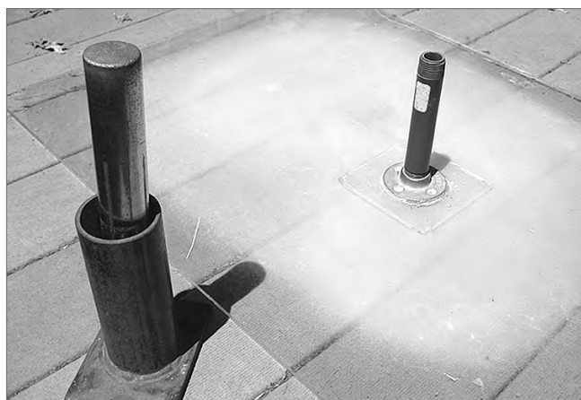
Metal cylinder for smashing quartz (left) and grinding glass (right) as used by Harald
