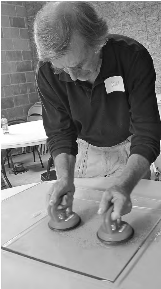
Grinding the quartz finer between two sheets of glass, again with a little water
